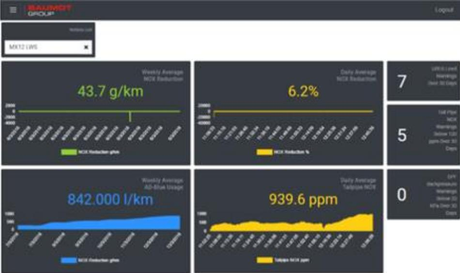
With HED’s integrated data logging tool any user can log CAN traffic and any other internal module parameters or statistics and export that data to any ftp or S3 bucket. With Baumot we have created a UI that links to that data for easy upload for analysis. HED can present this data in just about any format needed.
